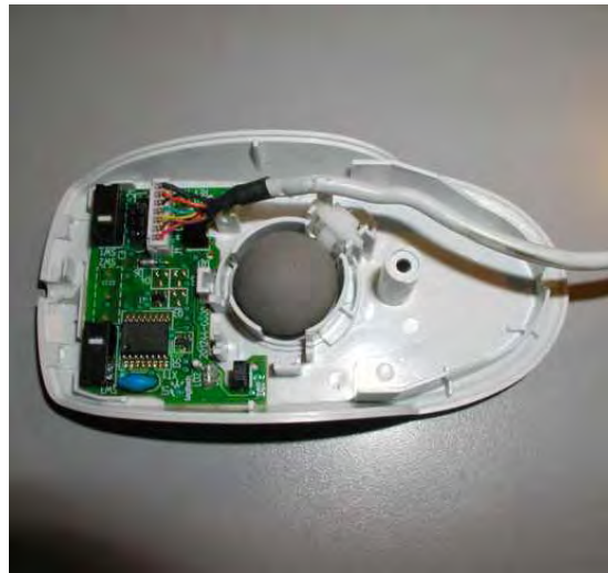
Under the Hood — Note Cable Reversed
